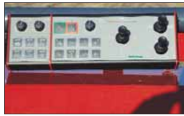
The control panel provides fingertip control of all functions from the tractor cab.
