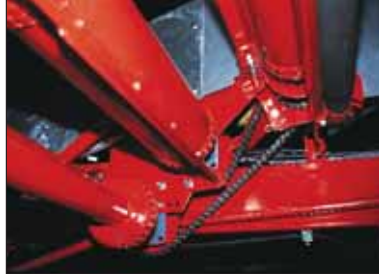
The 3 roller positive main web drive system facilitates easy changing of webs to suit different crop and field conditions.
