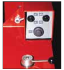
Control panel for: chassis and axial roller levelling and speed of the picking web from the picking platform.
